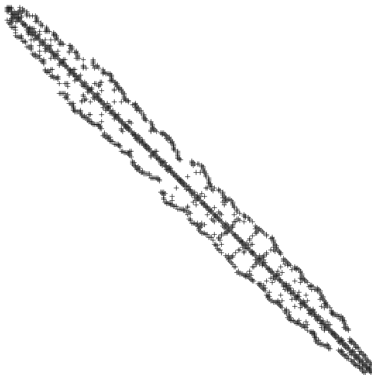
Figure 3: Sparsity of the FE Matrix After Renumbering
