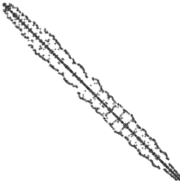
Figure 3: Sparsity of the FE Matrix After Renumbering
